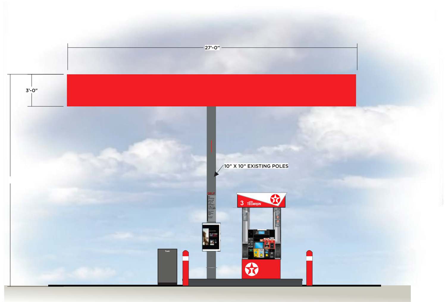
CANOPY 2 - ELEVATION SCALE: 3/16" = 1'-0"
