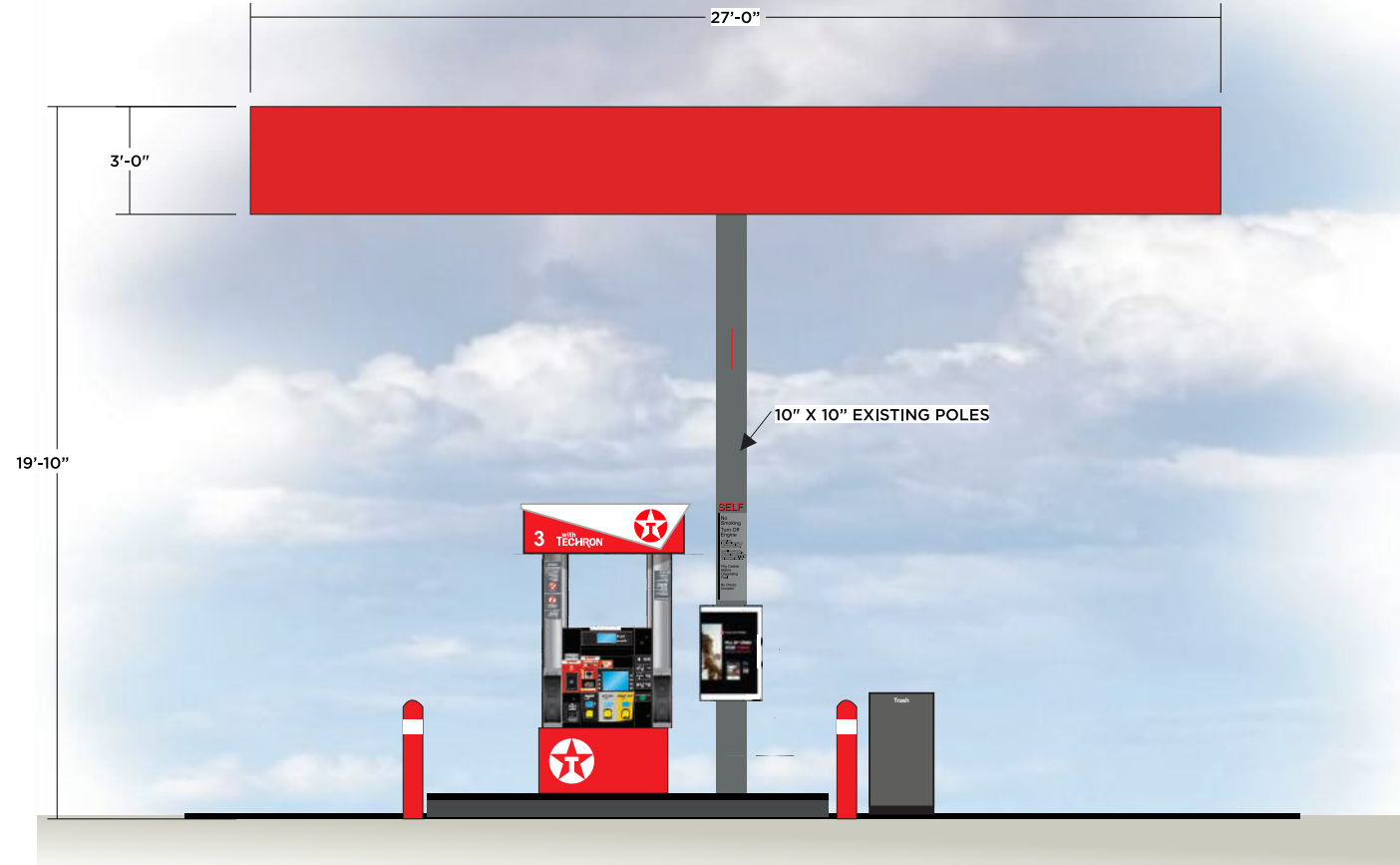
CANOPY 2 - ELEVATION SCALE: 3/16" = 1'-0"
